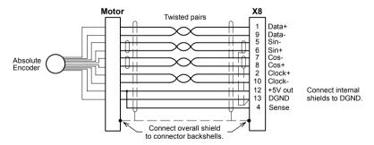
Figure 22 - Absolute encoder cable connections
